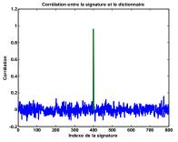
Fig. 1.6. Succeeded detection of a mark after correlation between extracted and decoded mark and the dictionary after Gaussian noise (0.03) attack. Correlation=0. 90
