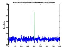
Fig. 1.7. Succeeded detection of a mark after correlation between extracted and decoded mark and the dictionary after image Compression of Quality 60. Correlation 0.83
