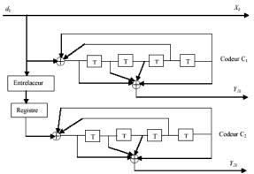
Fig. 1.4 Structural diagram of turbo coder
