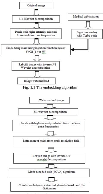
Fig. 1.2 The detection algorithm
